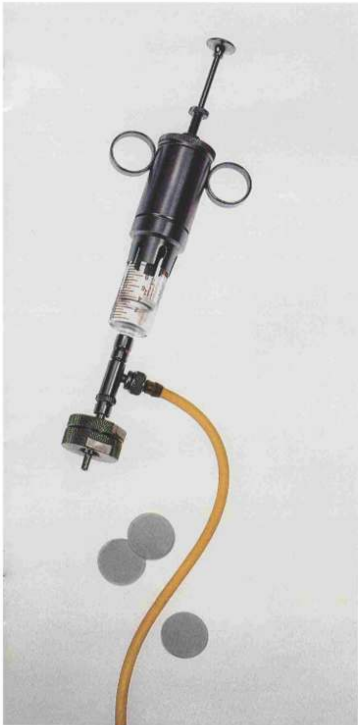
Pipette Assembly with filter holder
